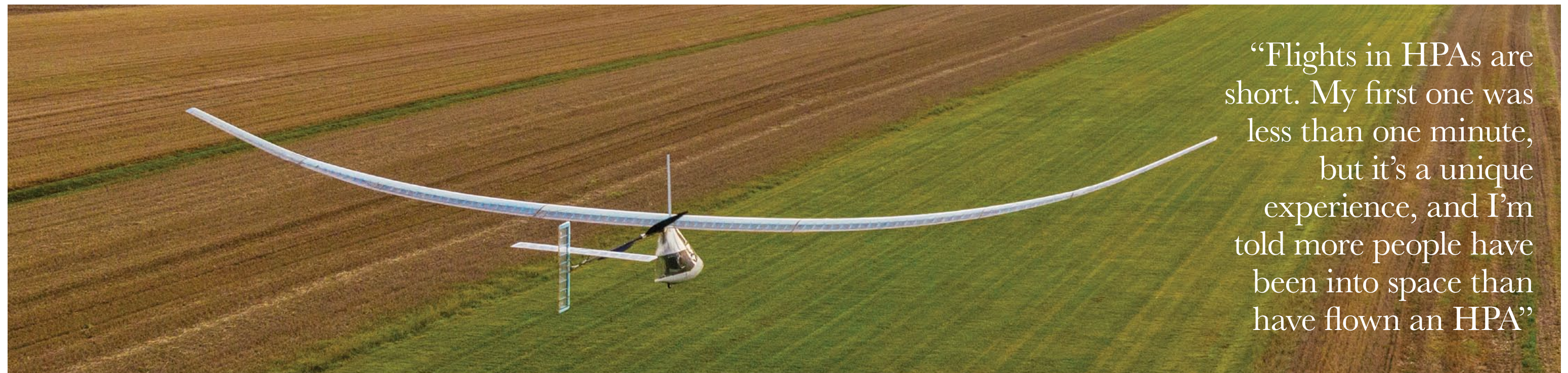
Right Fragile wings sag under their own weight prior to flight
