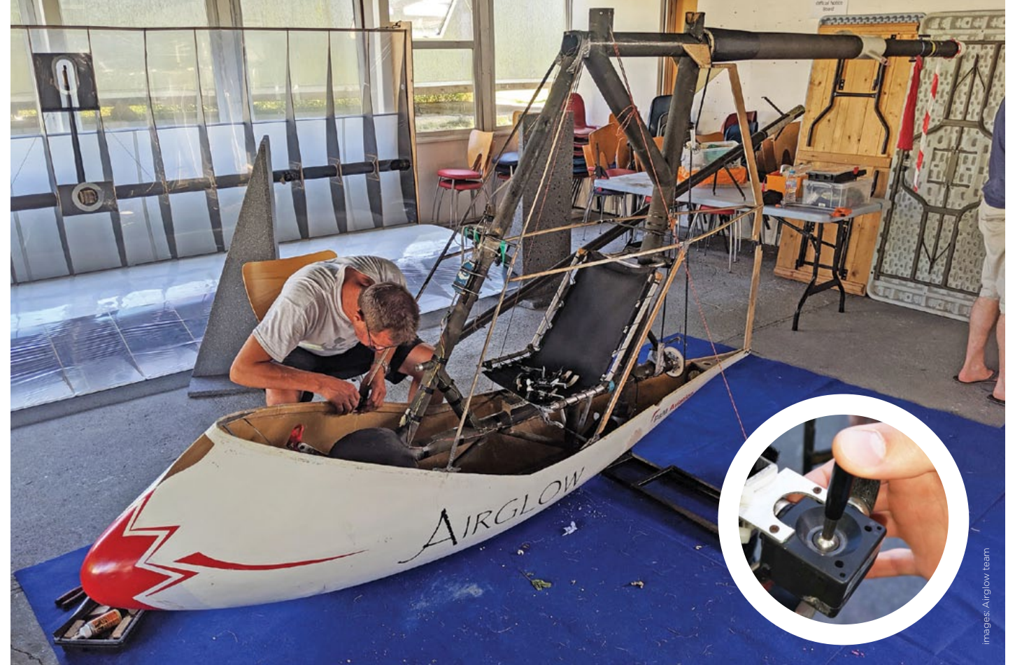
Above John Boyce reattaches the pod following some mid-competition maintenance. Note the long thin chain drive that runs behind the pilot's seat
