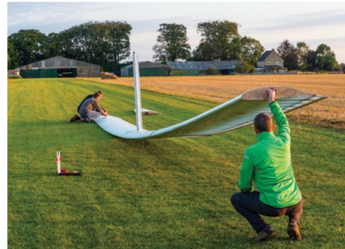
Opposite Team mates John Boyce, Sam Morley and Darren Arkright unload and assemble the fuselage Top and above The wing is made of seven separate sections, and a pre-bend load must be added to the centre three sections to attach the upper flying wires Left Each HPA is registered with the BHPFC Below The wing is attached to the top of the fuselage structure with two pins
