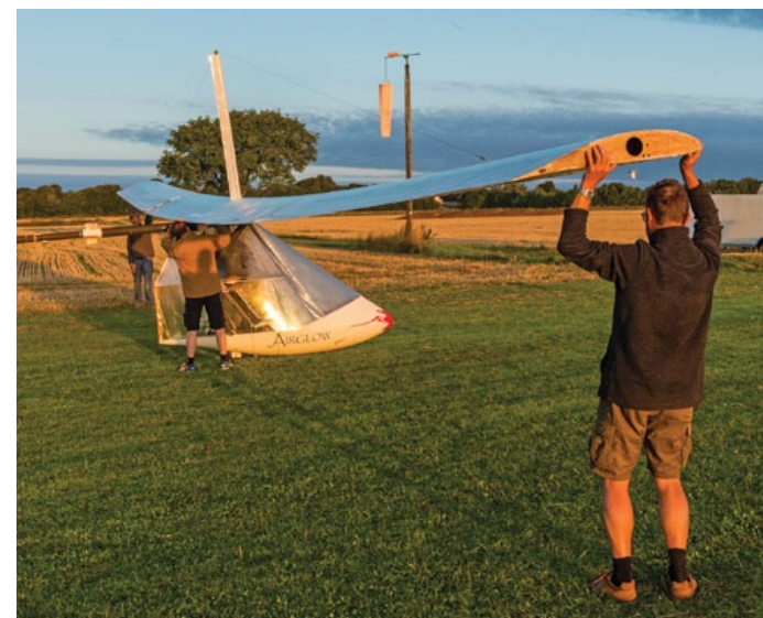
Opposite Team mates John Boyce, Sam Morley and Darren Arkright unload and assemble the fuselage Top and above The wing is made of seven separate sections, and a pre-bend load must be added to the centre three sections to attach the upper flying wires Left Each HPA is registered with the BHPFC Below The wing is attached to the top of the fuselage structure with two pins
